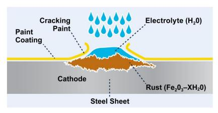
Figure 1 In order for the corrosion process to start, uncoated steel must be in contact with water and oxygen
